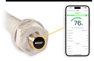
The Load Monitoring Fastener+® (LMF+) is a wireless system capable of automatically monitoring bolt preload during extended periods of operation. Transmission Dynamics are now offering a long range (LoRa) LMF+ with a wireless range of 4 km and an impressive battery life of up to 20 years, over the full industrial temperature range of -40 to +85°C.
